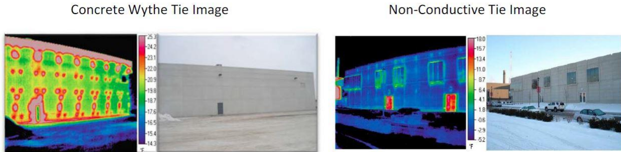
Fig. 2.5 – Thermal Image of panel with concrete tie vs. one with non-conductive Wythe-tie
